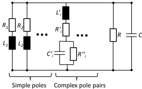
Figure 2: RLC equivalent circuit for the fit function
