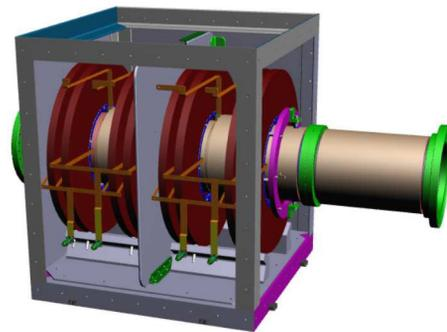
Figure 4: CAD model of the ESR cavity
