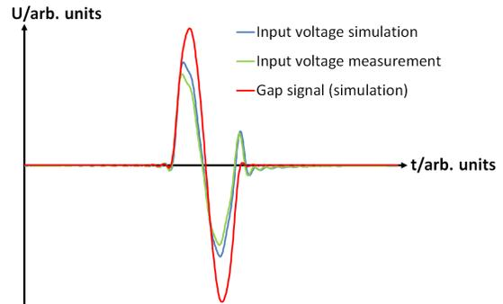
Figure 7: Input signals and resulting gap voltage
