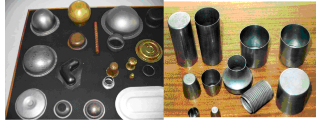
Figure 4: Examples of components produced by impact hydroforming at PTI NASB.
