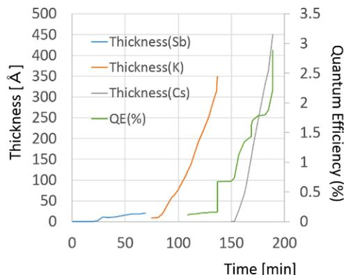
Figure 4: An example of cathode fabrication. The left and right vertical axes show thickness of each materials and QE measured with 405nm laser, respectively. The green, red, and yellow curves show thickness of Sb, K, and Cs, respectively. K and Cs evaporation was terminated when QE is saturated.
