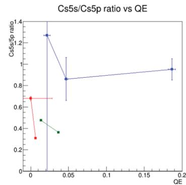
Figure 6: Cs 5s/ Cs 5p ration in CsK<sub>2</sub>Sb UPS spectra.
