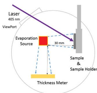
Figure 3; Schematical drawing of the evaporating chamber. The metal vapour was generated in two directions.
