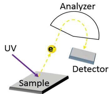
Figure 1: A schematic picture of UPS measurement. The kinetic energy of photo-electrons from a material with UV light is analysed with an electro-static analyser.
