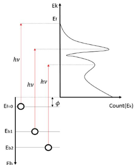
Figure 2: By measuring UPS spectrum (upper right figure), we can extract the band structure of material (lower left figure).
