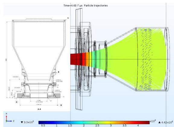
Figure 8: The collector: mechanical drawing (left), electron trajectories in the collector (right).
