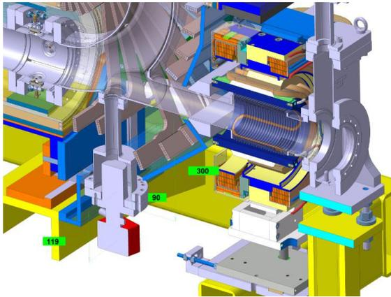
Figure 6: Integration of the vacuum pumping elements in the electron cooler.
