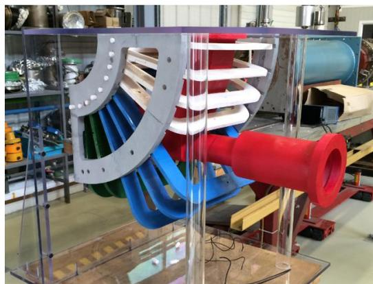
Figure 5: 3D print model of the toroid section.
