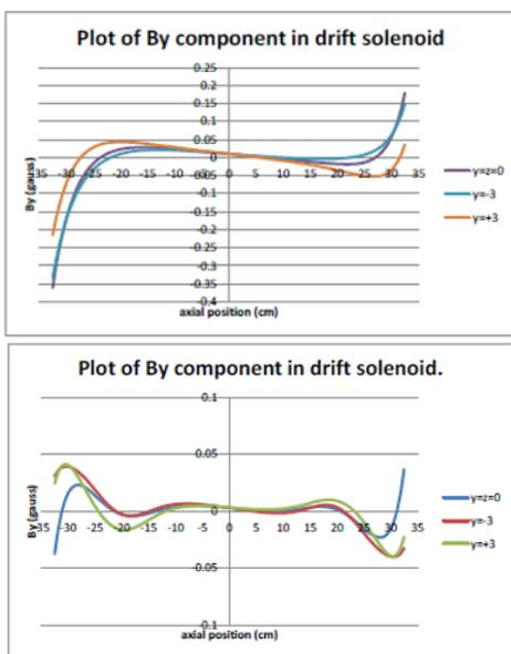
Figure 3: Plot of  $B_y$  along the drift solenoid without any correction (top) and with the fine-tune coils (bottom).
