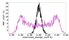
Figure 8: The bunch energy distribution at time t=0 (black line), and t=structure exit (pink line) after interaction with the laser.
