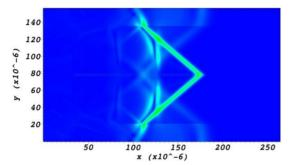
Figure 3: The electric field of the electron bunch travelling along the vacuum channel of the structure.
