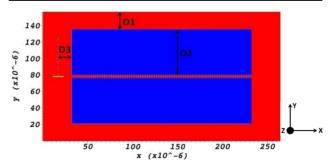
Figure 2: Model of a 100-period dual-grating structure in the VSIM code. The red area represents vacuum, the blue area dielectric material with a refractive index n=1.5, and the injected electron bunch is represented in yellow.
