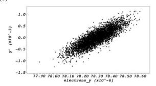
Figure 4: Transverse (y direction) phase space for the electron bunch at time t=0 (a), and t= structure exit (b)
