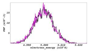
Figure 5: Bunch energy distribution at time t=0 (black line), and t= structure exit (pink line) without a laser, where PDF stands for probability density function.
