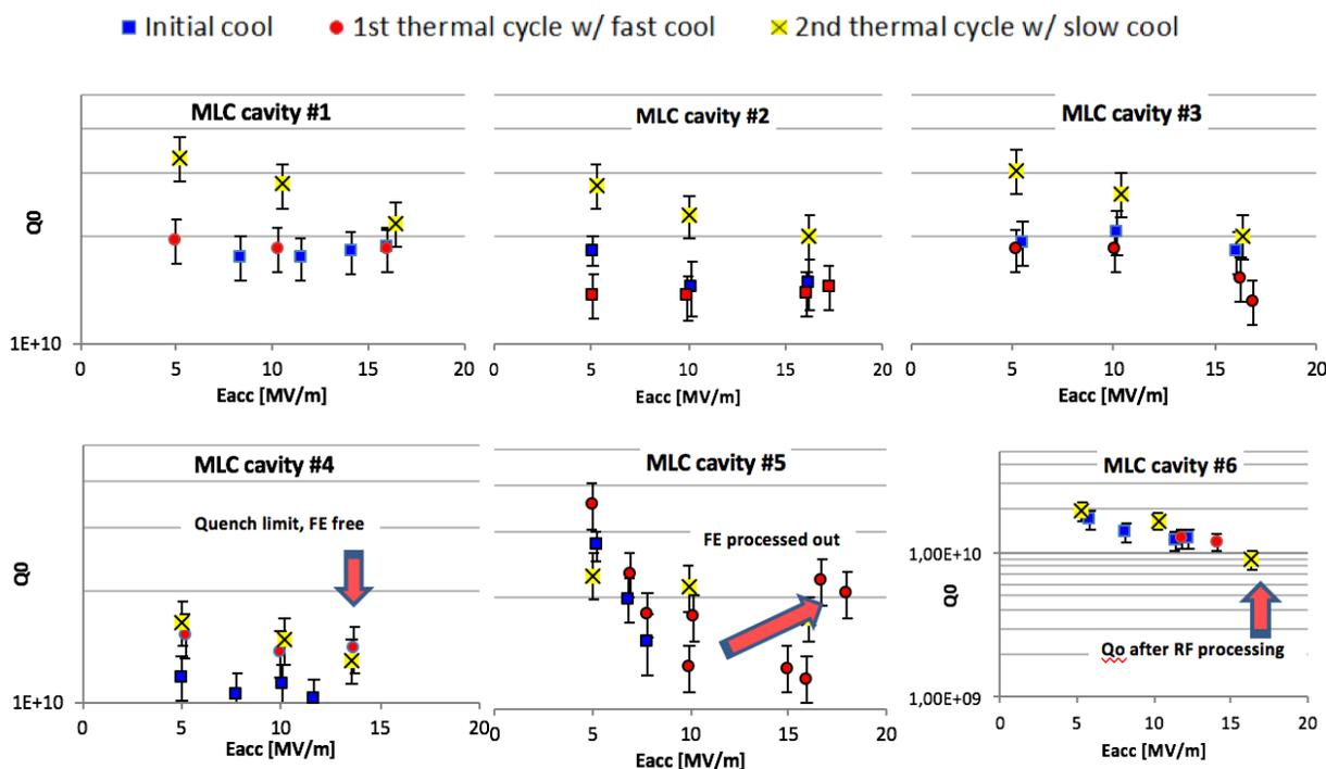
Figure 6: Summary of the cavity performance. All data were taken at 1.8 K. Two cavities had to be RF processed to increase the field and to remove field emission. Cavity #4 is still limited by an early quench, but administrative procedures (for now) prevented us from processing this cavity harder.
