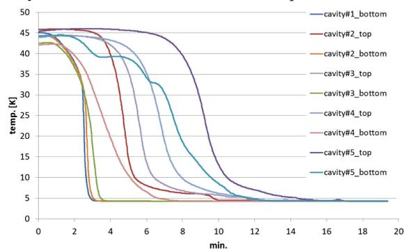
Figure 5: Cavity temperatures during the fast cool-down resulting in a speed of 0.5 K/min to 2 K/min, depending on how close the cavity was to the JT valve.
