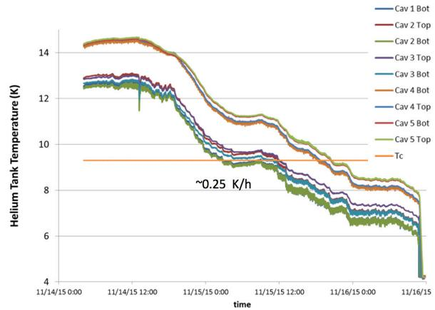
Figure 4: Slow cool-down cycle performed in order to measure cycle dependant impacts on the cavity performance. For the slow cool-down we were able to get 0.25 K/h relatively uniform over the cryo-module.
