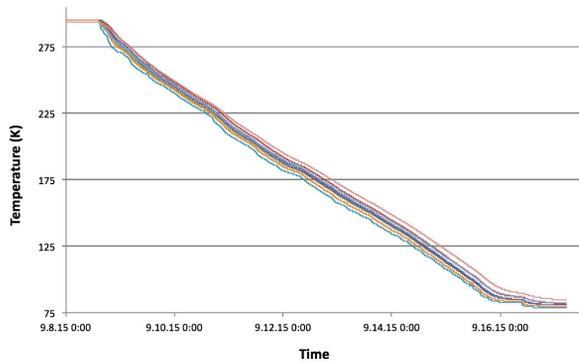
Figure 2: Temperatures on the thermal shield during the cool-down. Due to the design of the thermal shield the temperature spread across the shield had to stay below 20 K, leading to a cool-down rate of  $\sim 1.25$  K/h.
