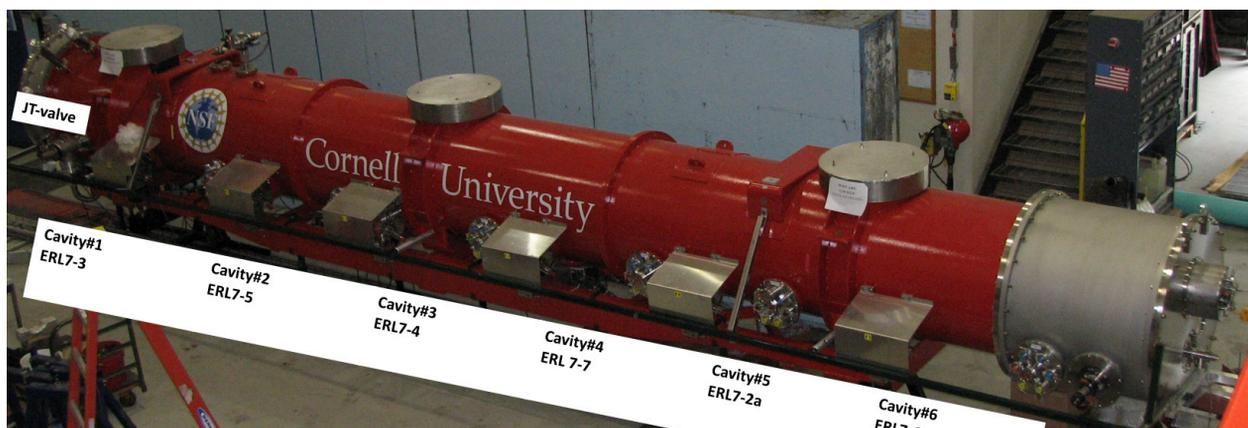
Figure 1: Cornell's Main linac cryo-module during the installation in Wilson Lab. Positions of the cavities are also depicted.
