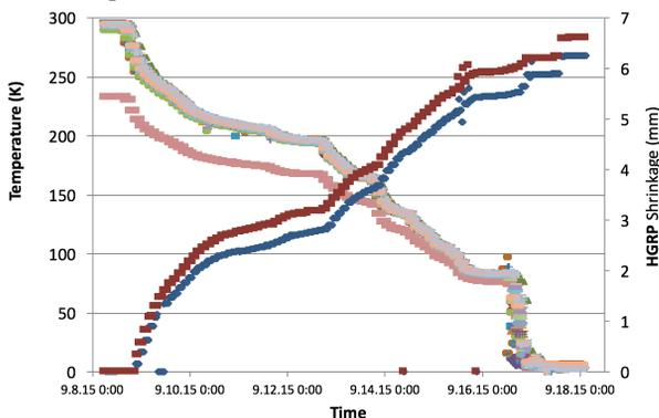
Figure 3: Movement of the outer (sliding) support posts: as the temperature of the HGRP goes down the posts move inwards. The movement was as expected.
