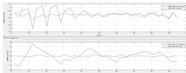
Figure 3: BPM's read-outs from horizontal (upper diagram) and vertical (lower diagram) planes for all 12 DBA magnets without any corrections (blue line) and with correction (red line).
