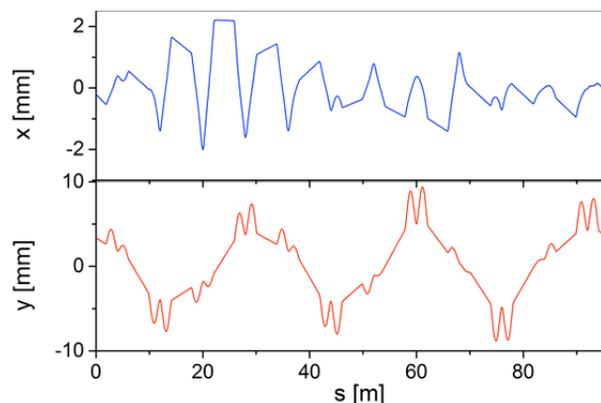
Figure 4: Simulated orbit around Solaris storage ring without any correction.
