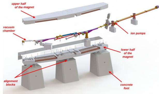
Figure 1: Double Bend Achromat Magnet (DBA) layout.
