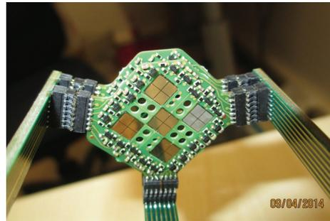
Figure 1: Diamond based mosaic detector which was located in front of the HADES target in a pion production beam time. An total area of  $14\text{ mm} \times 14\text{ mm}$  was covered. The first transistor based pre-amplification stage is located very close to the diamond material.
