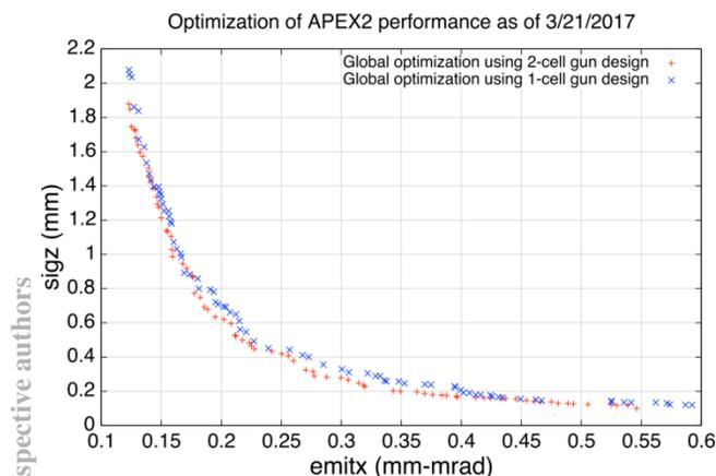
Figure 4: Pareto-optimal fronts showing the performance of APEX-2 using an injector layout based on two different gun design options.
