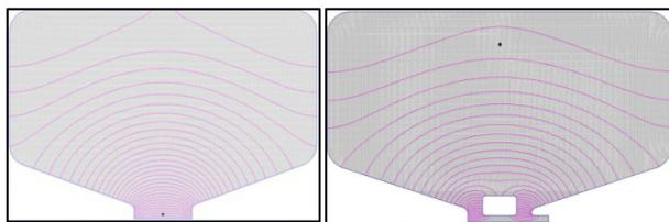
Figure 3: Superfish calculations showing the electric field geometry inside (half of) the cavity. Top: case of a single cell double reentrant nose cavity. Bottom: same design with the addition of a drift tube in the center of the gap.
