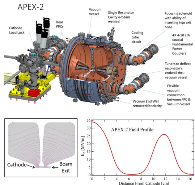
Figure 2: Top: CAD view of the conceptual design for a two-cell geometry of APEX-2 with its main components. Bottom left: Superfish calculation showing the electric field geometry in (half) the cavity. Bottom right: accelerating field intensity along the axis of the gun.
