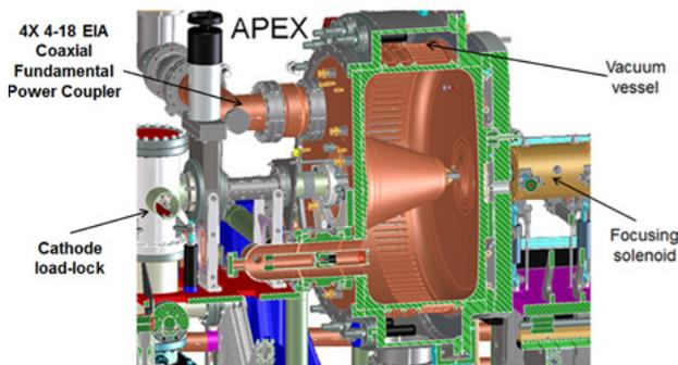
Figure 1: CAD cross-section view of the existing APEX gun with main components in evidence. The two main RF couplers and the vacuum plenum where up to 20 NEG modules can be located are visible. The photo-cathode is located on the tip of the nosecone and can be inserted/removed from the gun without breaking the vacuum by the vacuum loadlock system located in the back of the gun. The radius of the cavity is about 35 cm.
