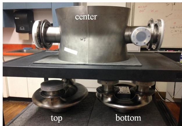
Figure 1: Cavity subassemblies.
