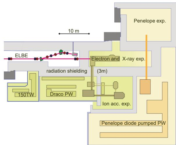
Figure 1: Floor plan of the upgraded HZDR ELBE center for high power radiation sources, illustrating the placement of the two PW lasers as close as possible to the dedicated target areas presently under operation or development (green: DRACO (Dresden Laser Acceleration Source), orange: PENELOPE (Petawatt energy efficient laser for plasma experiments)) and the connection to the beamline of the linear accelerator (red) with its user facility radiation sources (not shown) extending to the left.
