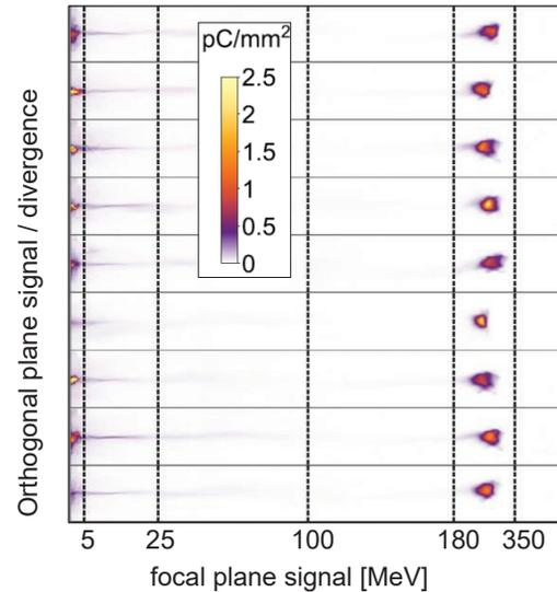
Figure 6: Spectrometer raw-data for 9 consecutive shots illustrating the stability of the peaked energy distribution at low medium energy background level. Typical charge per bunch is 250 pC (FWHM) in the peak at a relative bandwidth of 15%.
