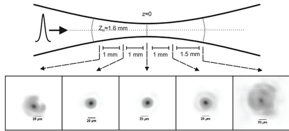
Figure 3: Development of the transverse intensity profile of the laser pulse in the vicinity of the focal spot generated with an F/20 off-axis parabolic mirror.
