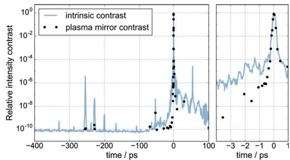
Figure 4: Intensity pulse contrast, measured with a scanning third order autocorrelator for the standard configuration (intrinsic) and behind a single stage plasma mirror (dots), highlighting the contrast improvement on the ps-scale.
