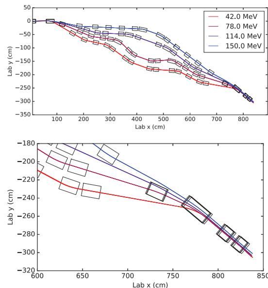
Figure 5: Layout of magnets for all four passes.
