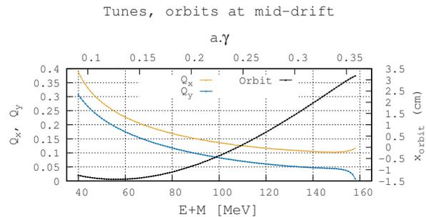
Figure 7: Energy dependence of the tunes in a CBETA cell defined using QF and BD 3D field maps, to replace the usual SBEND or MULTIPOLE optical elements.
