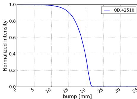
Figure 2: Intensity evolution during the scan of the amplitude of a three-corrector bump at location of QD.42510.
