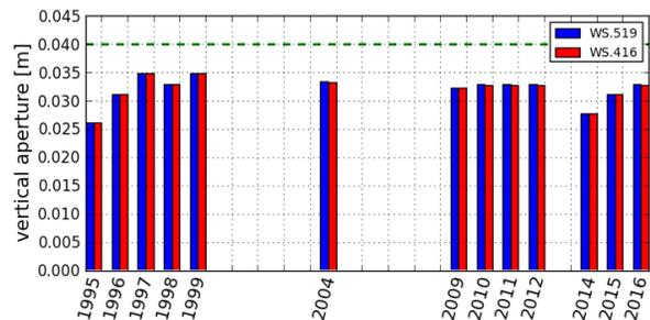
Figure 1: Result of global aperture measurement in the vertical plane with wire scanners 416 and 519 for the different SPS runs scaled by the beta function to the location of the internal beam dump TIDVG. The dashed green line indicates the aperture at the TIDVG minus 2 mm to account for the misalignment.
