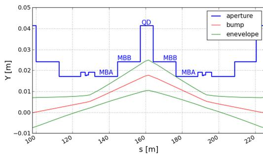
Figure 3: Mechanical aperture in the FODO cell of the SPS in the vertical plane with three-corrector bump and beam envelope. The bump will touch the aperture at the MBA to MBB or QD to MBB transition before reaching the QD aperture.
