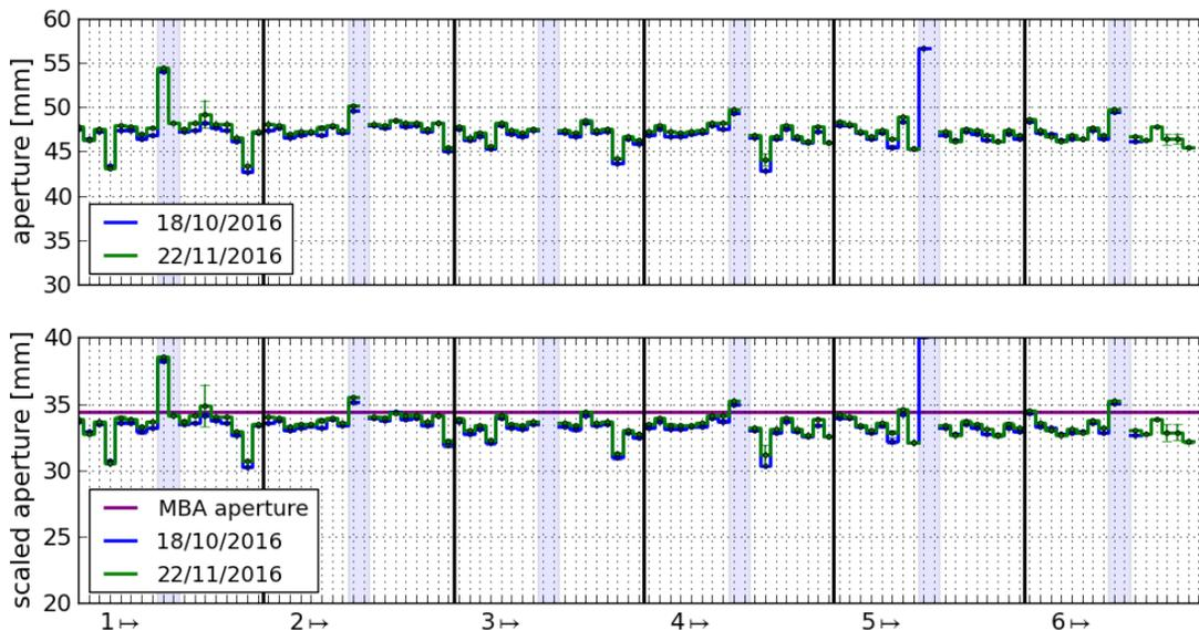
Figure 4: Total aperture measured at all defocusing quadrupole locations on 18<sup>th</sup> of October in blue and on 22<sup>nd</sup> of November in green. The numbers 1 - 6 on the bottom of the plot indicate the number of the corresponding sextant. The shaded areas correspond to the LSS. The lower plot shows the aperture measurements scaled to the location of the MBB-MBA transitions. The aperture of the MBA vacuum chamber is also indicated
