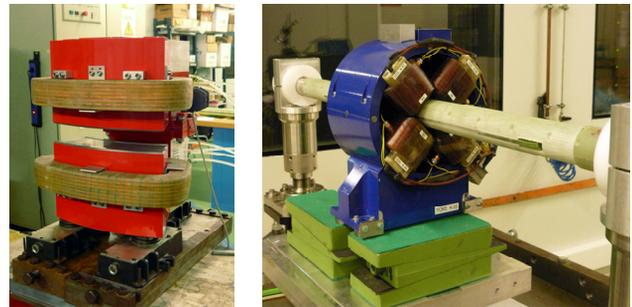
Figure 4: Image of ThomX dipoles (*left*) and quadrupoles (*right*).
