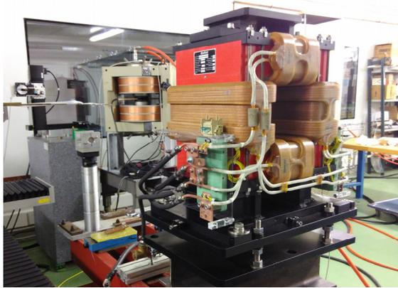
Figure 5: CNAO corrector on Hall probe bench at ALBA magnetic measurements laboratory.
