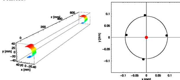
Figure 3: Procedure to determine the rotation axis of the coil. *Left*: Scan with the laser tracker of the surface of both ends of the coil. *Right*: Determined center of the coil at 4 different orientations (*black dots*) and reconstructed center of rotation (*red dot*).
