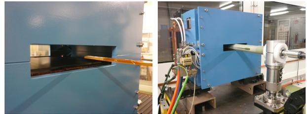
Figure 6: CLARA dipole magnet being measured with Hall probe (*left*) and rotating coil (*right*).
