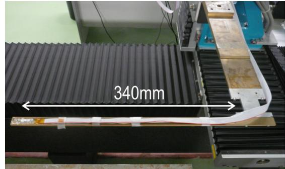
Figure 1: Image of long Hall probe for the measurement of magnets without lateral access.
