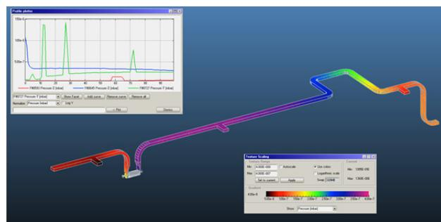
Figure 4: Single line Molflow vacuum simulation plot.
