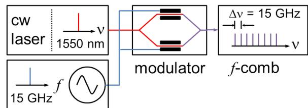
Figure 1: Simplified scheme for the generation of a frequency comb using a continuous wave (cw) laser at a telecom frequency, a radio frequency source at e. g. 15 GHz, and a modulator based on an electro-optical material such as  $\text{LiNbO}_3$  and individual modulation of each arm in a Mach-Zehnder interferometer. The resulting frequency comb with comb tooth spacing of 15 GHz can be further modified for applications, e. g. compression to a short sub-picosecond terahertz pulse.
