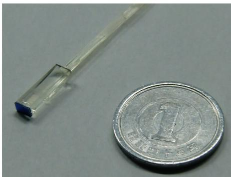
Figure 3: Electro-optical probe integrated with 16 fiber-based channels suited for telecom frequencies around 1550 nm and Japanese 1-yen coin with a diameter of 20 mm and a thickness of 1.5 mm for size comparison.
