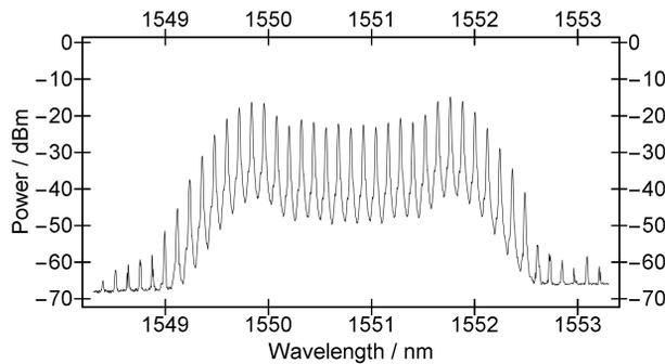
Figure 2: Experimental result of frequency comb generation using a telecom single-frequency continuous wave laser and a LiNbO<sub>3</sub> modulator operated with a radio frequency of 15 GHz .
