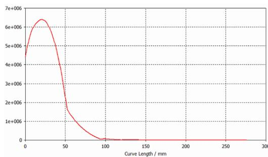
Figure 3: Simulated electric field along cavity axis.
