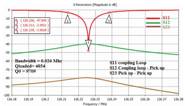
Figure 5: Frequency domain simulation results.
