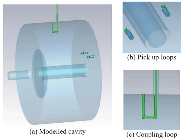
Figure 4: Simulation model in frequency domain solver.
