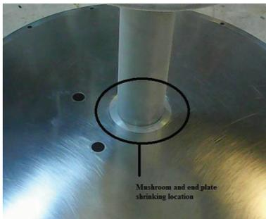
Figure 6: Mushroom part connected to the sidewall by shrinking method.
