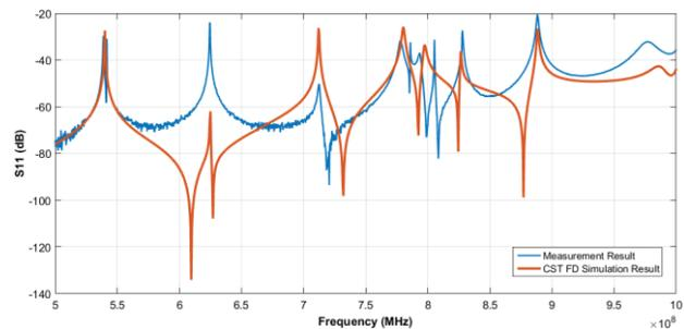
Figure 10: Higher order modes spectrum between 500 to 1000 MHz
