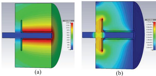
Figure 2: simulated fields profiles of  $TM_{010}$  mode at 126.2 MHz (a) Magnetic (b) Electric.
