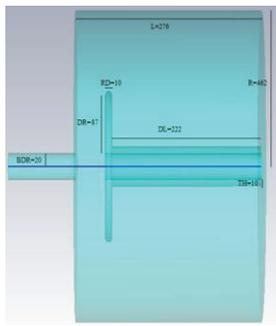
Figure 1: Simulation model of the cavity with optimized dimensions
