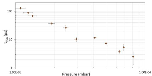
Figure 8: Evolution of the beam rise time when the chopper is switched-off as function of the residual gas pressure (Kr injection).
