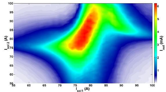
Figure 3: Transmission map ( $P = 1.1 \cdot 10^{-5}$  mbar, collimators aperture = 48 mm).
