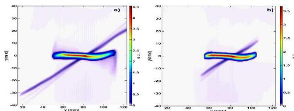
Figure 2: Beam distribution in the vertical phase space measured at the middle of the LEBT: a) without collimation, b) with collimation
