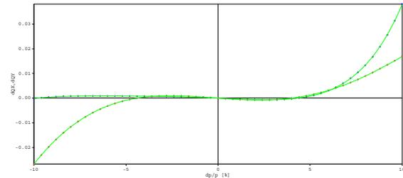
Figure 7: Chromatic octupoles help to reduce deviation of horizontal and vertical tunes to  $\delta Q_{X,Y} \leq 0.03$  for off-momentum particles even at  $\delta p/p = \pm 10\%$ . Strength of octupoles was limited to minimize reduction of ring acceptance.
