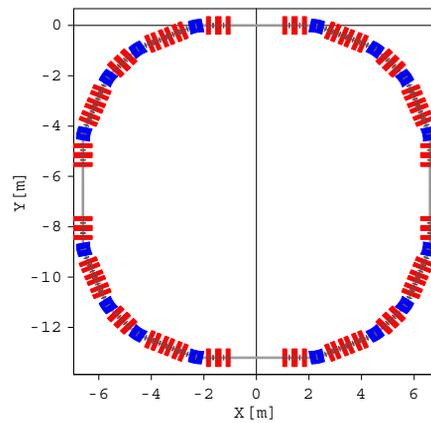
Figure 2: Four fold symmetry model of Very Large Acceptance compact Storage Ring fitted into FLUTE bunker.  $22.5^\circ$  bends are depicted in blue, multipole focusing magnets in red, elements located between quads are not shown [5].
