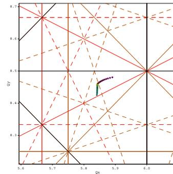
Figure 6: Tune diagram. Combination of sextupoles and chromatic octupoles helps to localize and wrap up foot-print of chromatic tune deviation for particles with momentum offset of up to  $\delta p/p \leq \pm 10\%$ .
