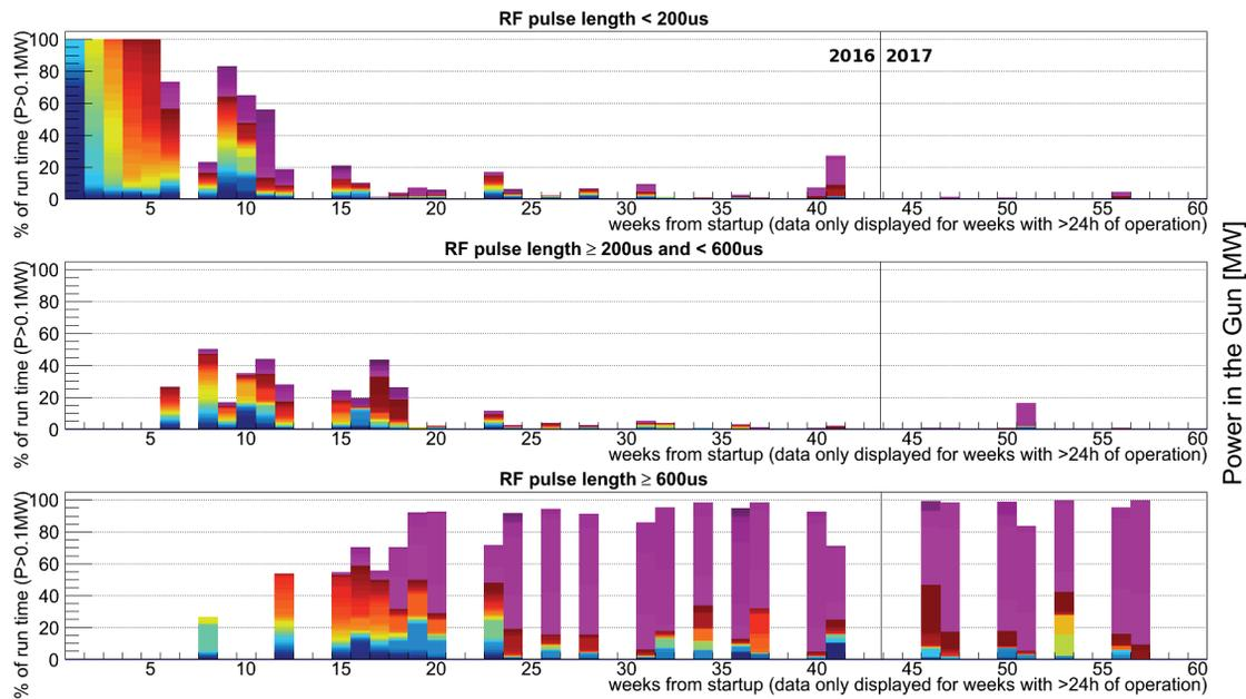
Figure 2: Weekly percentage of Gun 4.6 operation time spent at different RF pulse lengths. The color code provides further information about the time spent at different power levels. Weeks with less than 24h operation time are not shown.
