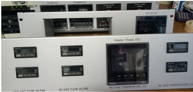
Figure 3: Front panel for the new Omron PID controller.
