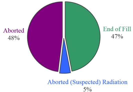
Figure 5: Physics beam aborts in 2016: due to failures (purple), due to radiation effects (blue) or triggered intentionally by operators (green).
