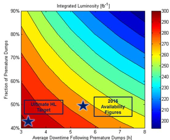
Figure 7: HL-LHC integrated luminosity production evolution as a function of machine availability.
