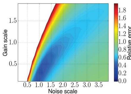
Figure 5: Relative difference between the measured increase of the emittance growth rate with the predictions of the weak-strong model, averaged over all data points of the scan with largest beam-beam tune shift for different relative errors on the ADT gain and noise amplitude.
