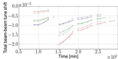
Figure 2: Beam-beam tune shift computed based on measured bunch intensities and emittances during each step of the experiment. The first two set of lines show the first cycle, the others represent tests performed in a single cycle, varying different machine settings. The blue, green and red lines correspond to low, medium and high intensity bunches respectively. The solid and dashed lines correspond to colliding bunches with full ADT gain and reduced gain respectively.
