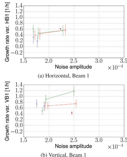
Figure 6: Variation of the emittance growth rate when introducing noise, w.r.t. the emittance growth rate observed in absence of artificial noise. The color code is identical to previous figures, the crosses indicated the results obtained in the second last scan (minute 240 to 270 in Fig. 2) with a chromaticity reduced to 10 units. The dots indicate the last step, with a chromaticity reduced to 5 units.
