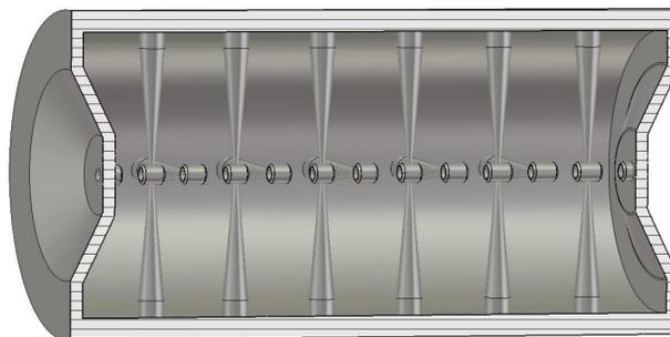
Figure 8: Sectional view of CH-cavity number 9.
