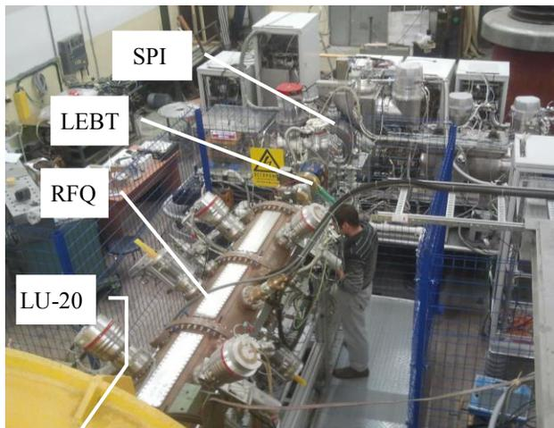
Figure 6: Source of Polarized Ions mounted on the HV terminal and RFQ connected to the LU-20
