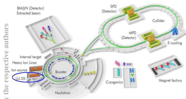
Figure 1: NICA complex. Proton, light and polarized ion linac LU-20 with new RFQ injector is marked.
