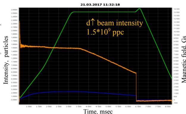
Figure 7: Cycle diagram for polarized deuteron beam during acceleration and slow extraction: orange line - intensity, green line - main magnetic field.
