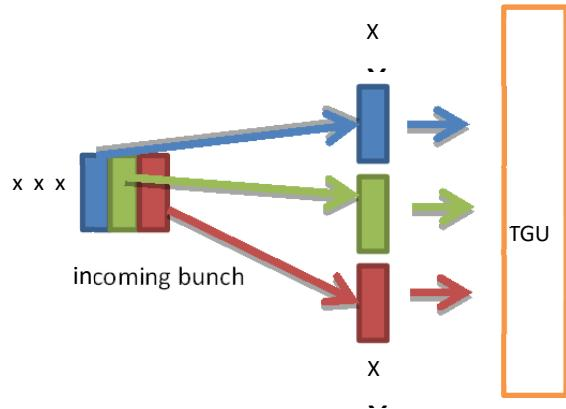
Figure 6: Example for an arrangement for producing coherent radiation. The incoming beam is split by the dog-leg, described by Fig. 4. The thickness of the slices define when a SASE or seeding procedure is required.
