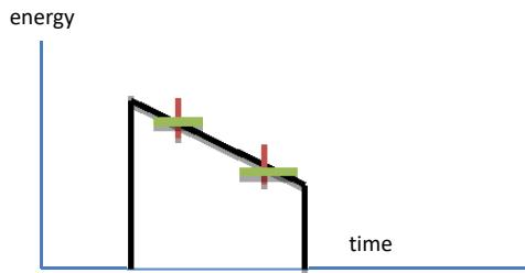
Figure 5: Schematic picture showing both correlated (black lines) and uncorrelated energy spread (red lines). The uncorrelated energy spread adds photons from a larger area (green) and increases the length of the photon train produced by the TGU. Fortunately the high correlated energy gradient (36 MeV in this example) limits this effect.
