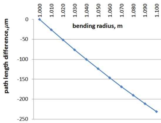
Figure 3: Path length differences in  $\mu\text{m}$  for particles with an energy difference of up to 10 % energy deviation bent by a 20 cm 1T magnet. Beam energy: 300 to 330 MeV. This curve shows the nonlinearities in the length already described in equation (2). Since the trajectories are locally separated the trajectory length can be corrected by additional magnets (not discussed in this paper). Figure 4 shows one possibility (among several other) how this can be done.
