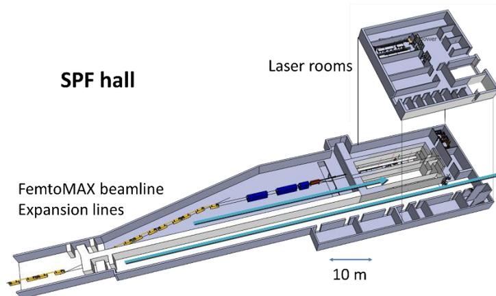
Figure 2: The existing SPF hall, the installed second bunch compressor and the FemtoMAX beamline. Blue arrows indicate tentative locations of the SXL.
