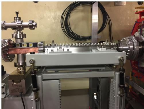
Figure 7: Stripline kicker with 6 mm full aperture between the striplines installed in the ALS.
