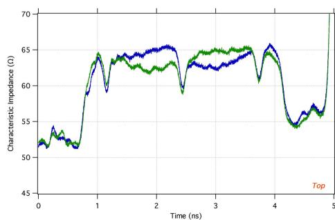
Figure 6: TDR measurements of the top and bottom striplines of the kicker. In the measurements, only one electrode is excited. The nominal impedance for that case is about 64 Ohms.
