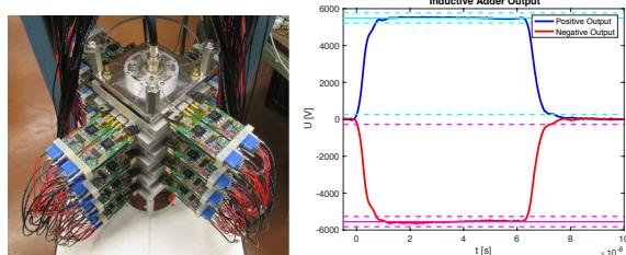
Figure 3: (Left) Full assembly (8 stages) of inductive adder. (Right) Voltage output of inductive adder at 105% of nominal setpoint.
