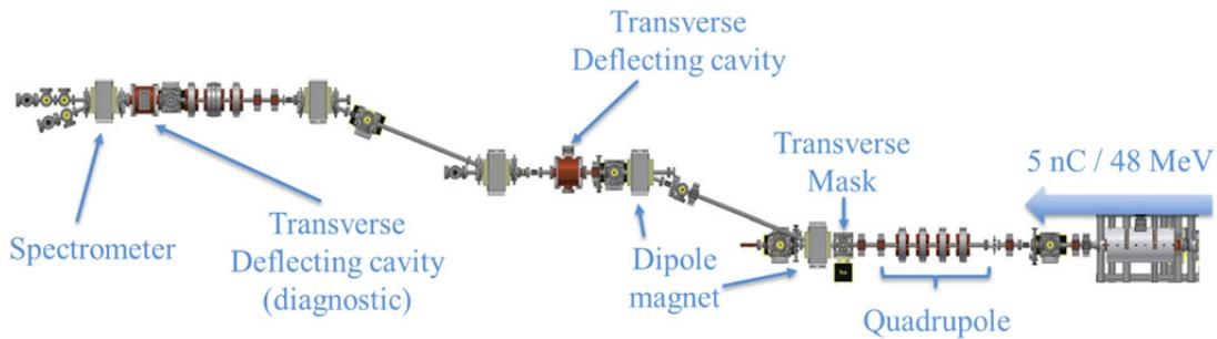
Figure 4: Schematic of the Emittance Exchange beamline, showing the two doglegs, two deflecting cavities, dipole and quadrupole magnets, as well as the position where masks are inserted to shape the transverse profile of the electron bunches. These customized transverse shapes can then create the desired longitudinal charge distributions.
