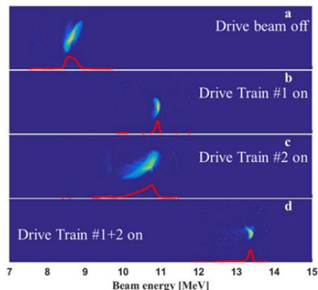
Figure 3: Four images of the spectrometer YAG screen, showing the witness beam energy under four different conditions: (a) without the propagation of any drive beams; (b) with drive bunches propagating through stage I only; (c) with drive bunches propagating through stage II only; (d) with drive bunches propagating through stages I and II.
