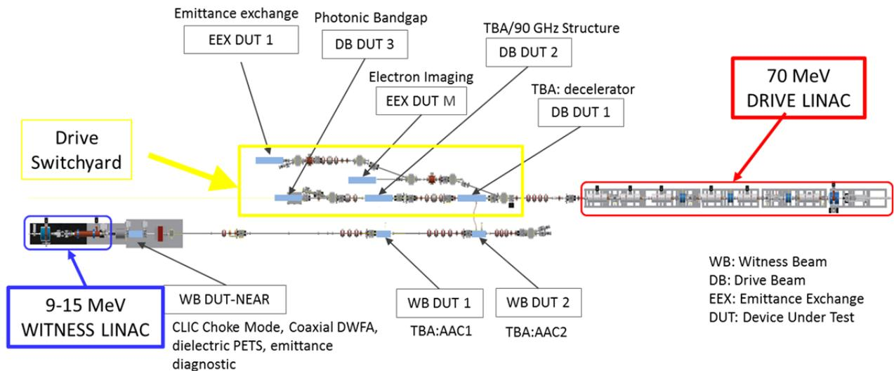
Figure 1: Schematic of the AWA beamlines, showing the two independent linacs and the experimental area where a large number of experiments have been carried out recently. witness beam accelerating structure, by means of a waveguide.
