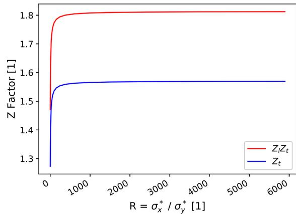
Figure 1: Transverse and total correction factors  $Z_t$  and  $Z_c = Z_l Z_t$  versus  $R = \sigma_x^*/\sigma_y^*$ .
