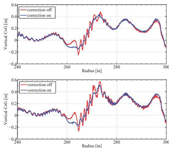
Figure 8: Result of radial probe measurements, showing that the resonance correction works well for reducing the amplitude of vertical oscillations coupled from the other centering errors due to detuned HC2's phase (upper) and amplitude (lower).
