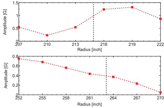
Figure 3: The  $B_r$  1st harmonic errors that exist in TRIUMF base field around the coupling resonance (indicated with the vertical dash-lines).
