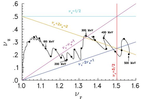
Figure 2: The TRIUMF cyclotron tune diagram, showing three passages through the coupling resonance  $\nu_r - \nu_z = 1$ .
