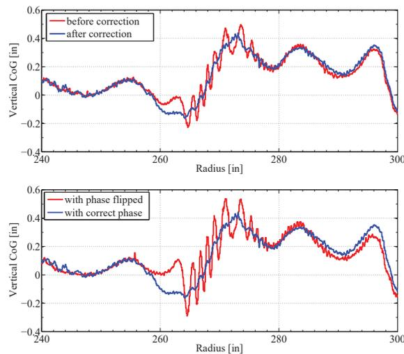
Figure 7: Result of radial probe measurements, showing the beam vertical oscillation amplitude significantly reduced after correction of the coupling resonance, where a coherent radial centering error of the beam orbit was intentionally introduced by detuning the deflector's high voltage. The flipped phase manifests the correct phase.
