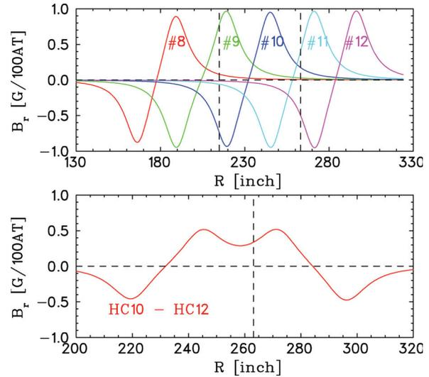
Figure 4: (Top)  $B_r$  component in the geometrical median plane due to harmonic coils HC8 to HC12. The 2 vertical dash-lines indicate where the resonance occurs. (Bottom)  $B_r$  due to HC10 combined with HC12, needed for the correction of the resonance occurring at  $\sim 291$  MeV (the vertical dash-line).
