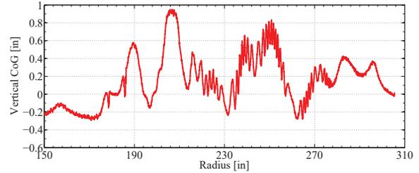
Figure 1: The radial probe measured vertical beam centroid vs. radius, showing the fast oscillations of an amplitude  $\sim 0.2$ " due to the radial-vertical coupling resonance.
