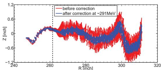
Figure 6: Result of simulation for the accelerated orbit, showing the trajectory of a single particle in the  $(r, z)$  space turn by turn for a number of turns until it gets to the extraction, before and after correction of the coupling resonance.
