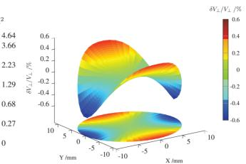
Figure 4: The relative transverse voltage variation in the circular region of radius 10 mm around the axis of the cavity forDesign-V.Thebeamtraversealongthez-axis.
