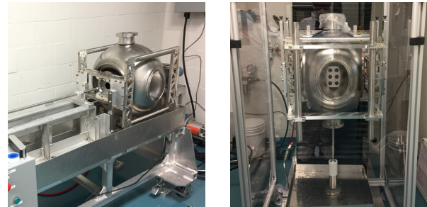
Figure 4: Horizontal HPR (left) and vertical HPR (right).
