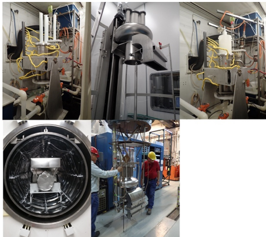
Figure 2: The 500MHz cavity on the BCP stand (top left), on the HPR stand in the clean room (top middle), on the VEP stand (top right), in the vacuum furnace (bottom left), and on the vertical test stand (bottom middle).
