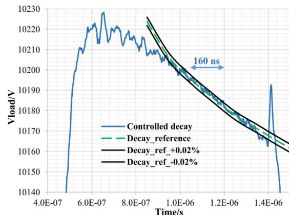
Figure 4: Simulated optimum waveform for the CLIC DR extraction kicker (green) with  $\pm 0.02\%$  stability margins (black), and an average of 100 measured pulses (blue) of the prototype inductive adder.
