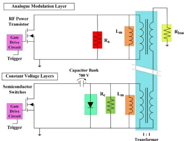
Figure 1: Schematic of an inductive adder with a single constant voltage layer with core loss resistance  $R_c$  and magnetizing inductance  $L_m$ , and with an analogue modulation layer with modulation resistance  $R_a$ , magnetizing inductance  $L_m$  and an RF power transistor.
