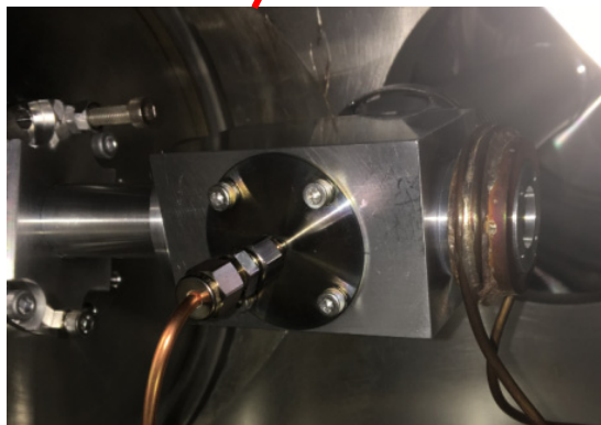
N2 gas jet system actually installed
