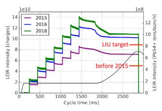
Figure 1: Evolution of the intensity along the LEIR cycle including Run 1 performance records.
