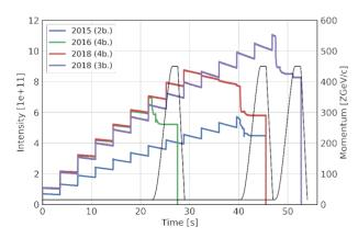
Figure 3: Intensity (in charge) from the beam current transformer along the SPS cycles for the ion runs from 2015 to 2018. The number of bunches per PS batch is indicated in the legend. The momentum along the cycle is also shown.
