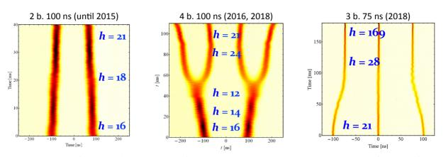
Figure 2: Overview of beam production schemes for Pb-ions in the PS used during Run 2: the waterfall plots of the wall current monitor are shown at an intermediate energy plateau for the 2 bunches spaced by 100 ns (left) and the 4 bunches spaced by 100 ns (center), while the 3 bunches spaced by 75 ns are obtained by batch-compression at flat-top (right).
