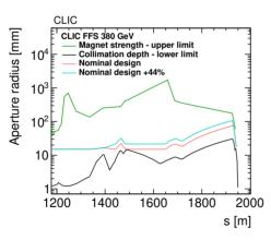
Figure 5: Extended apertures distribution in the Final Focus System at 380 GeV.
