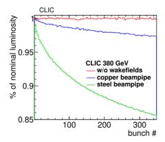
Figure 2: Luminosity distribution along the bunch train with copper and steel beampipes in CLIC BDS at 380 GeV.
