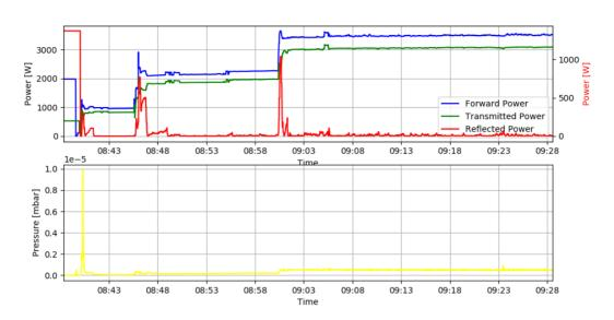
Figure 3: Measured power and pressure data for the commissioning of CH 1 up to 3 kW.
