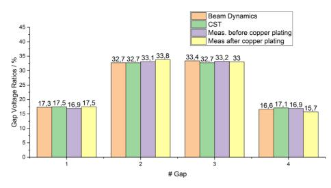
Figure 5: Comparison of the gap voltage ratios of CH 2.
