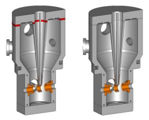
Figure 1: Comparison of a QWR with allowance (marked in red on the left picture) and without allowance.
