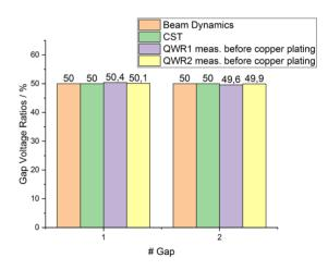
Figure 2: Comparison of the gap voltage ratios for QWR 1 and OWR 2.
