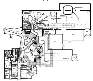
Figure 1: Preliminary layout of the ISOLDE target area with beam lines to the experimental hall and the implantation of the ISR.
