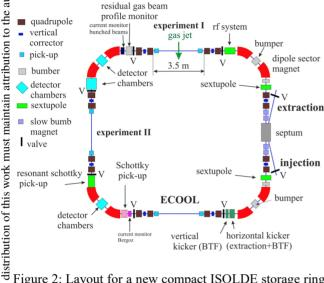
Figure 2: Layout for a new compact ISOLDE storage ring by M. Grieser, MPI-K Heidelberg
