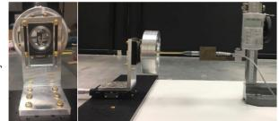
Figure 5: Low-cost permanent quadrupole magnet test apparatus (Oxford).
