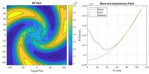
Figure 2: Measured magnetic field map (left), and resultant average field vs. the isochronous field (right).
