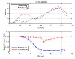
Figure 4: Magnetic field 1st harmonic amplitudes (top) and beam transmissions before and after the shimming.
