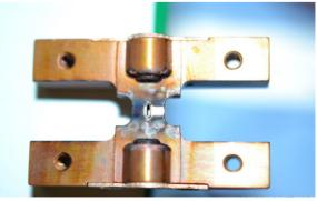
Figure 5: The Ion-12SC cold-cathode low power internal PIG ion source.
