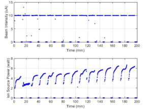
Figure 9: Beam intensity on target (top) and ion source power (bottom) of production runs in a day at UM.
