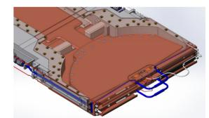
Figure 6: New direct water-cooled dummy dee circuit for Ion-12SC.
