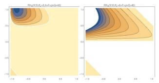
Figure 4: RH<sub>4</sub> in  $\Psi,\Theta$  plane. Left: cream-coloured areas stable. Right: white areas stable. Unloaded regime  $\tau_c\Omega$ =Q (mechanical). Large control loop gains. Stable area reduced compared with Fig. 3.
