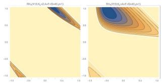
Figure 2: RH<sub>4</sub> in  $\Psi$ , $\Theta$  plane. Cream-coloured areas stable. Heavily loaded regime  $\tau_c\Omega$ =1. Large control loop gains. Stable area increased, compared with Fig. 1.
