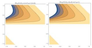
Figure 1: RH<sub>4</sub> in  $\Psi$ , $\Theta$  plane. Coloured areas unstable. Classic oscillatory condition is upper left quadrant: high frequency side Tan $\Psi$ <0 and Sin $\Theta$ >0. Heavily loaded regime  $\tau_c\Omega$ =1. Small control loop gains.
