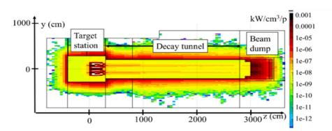
Figure 3: Power density deposited in the whole system.
