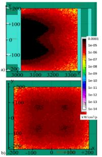
Figure 4: Longitudinal (a) and transversal (b) distributions of the power densities in the dump.
