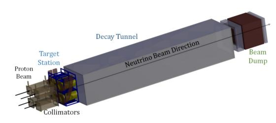
Figure 1: Schematic view of the target/horn station, the tunnel and the beam dump.
