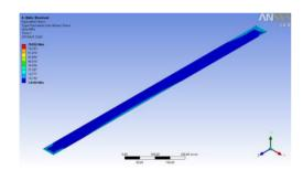
BY 3.0 licence ( $\odot$  2019). Any distribution of this work must maintain attribution to the Figure 2: The equivalent (von-mises) stress of Ti foil strip at 313K under pretension of 50N.
