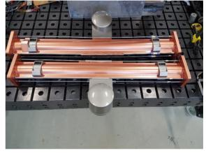
Figure 5: Short prototypes with pumping domes, Matsumoto-Ohtsuka-type flanges, and dummy BPM block.
