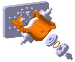
Figure 4: Exploded view of one BMP block, with electrodes (courtesy M. Gil Costa, CERN).
