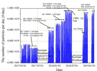
Figure 2: The change in RCS output power with respect to time.
