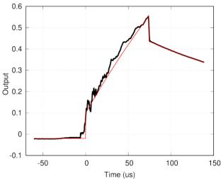
Figure 5: Best fit function (red) for full-aperture bunch monitor output waveform (black) in Fig. 4, based on the assumption of rectangular input.
