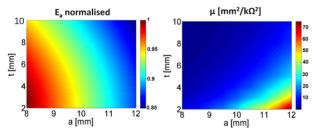
Figure 1: Normalized axial electric field and  $\mu$  parameter as function of the iris radius and the iris thickness.
