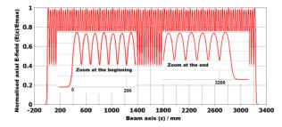
Figure 3: Normalized axial E-field along the structure.
