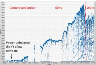
Figure 9: Conditioning plots: Peak power in MW vs. number of pulses for power splitter (top) and phase shifter (bottom).
