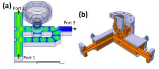
Figure 1: Variable RF splitter HFSS simulations (a) and general view of mechanical design (b).
