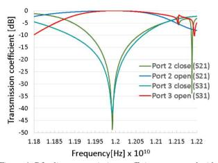
Figure 4: Rf splitter transmission coefficients measured with VNA.
