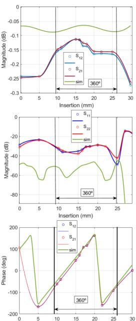
Figure 7: RF phase shifter transmission coeff. (top) reflection coeff. (middle) and transmission phase variation (bottom) vs. piston position from measurements and simu-(bottom) vs. piston position from measurements and simu-
